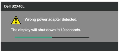
To avoid damage to the unit, user is strongly advised to use the original power adapter that comes packaged together with the monitor.
